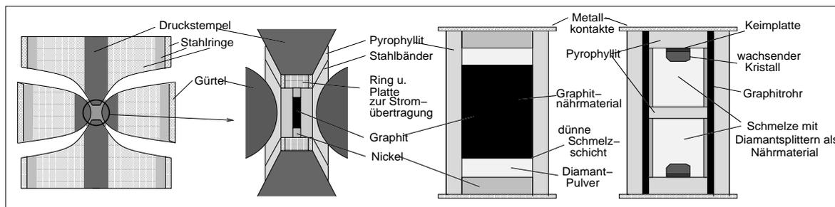
Belt-Apparatur zur Diamantsynthese
